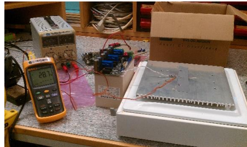
Figure 8.9.4: Heat sink temperature tripping test 28.7 °C, circuit has not tripped
