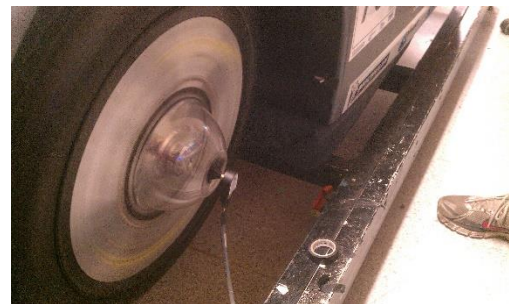
Figure 8.10.2.2: S1 taped to wheel with plastic cup testing
