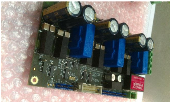
Figure 4.3.5.3: Inverter circuit board with components mounted, top view
