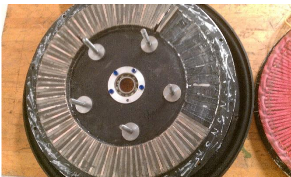
Figure 8.1.1: 2013 axial flux motor loose magnets on rotor plate 1
