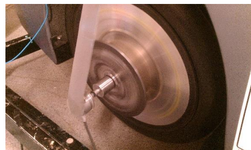
Figure 8.10.2.3: ROD 420 taped to test rig motor axle adapter testing
