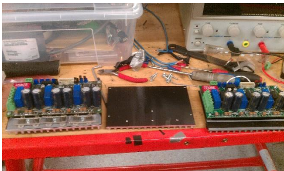
Figure 4.3.6.3: All of the three different inverter circuit boards under production
