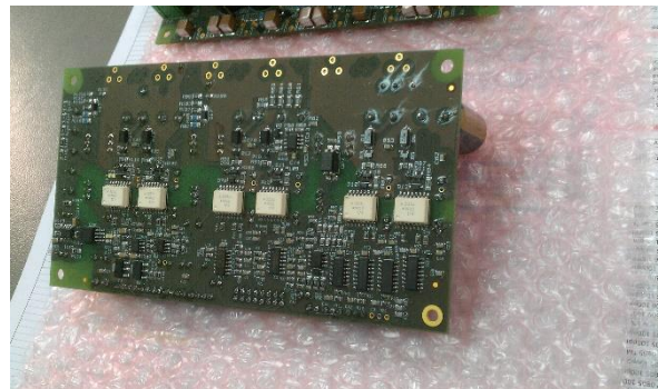
Figure 4.3.5.4: Inverter circuit board with components mounted, bottom view
