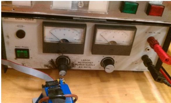
Figure 8.4.3.11: DC source, B02-0389, providing armature current to the DC machine
