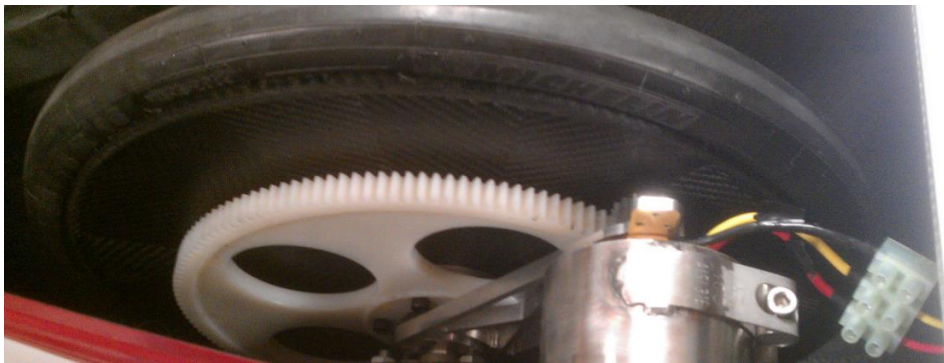
Figure 3.4.2.1: Motor mount and gear on the back wheel of the prototype vehicle
