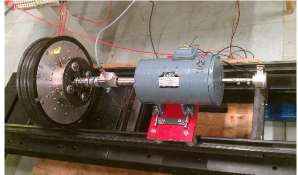
Figure 8.4.2.2: Test bench mechanical system with 2011 axial flux motor mounted to the rig, picture angle 2
