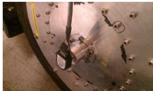
Figure 8.10.2.7: S1 connected first encoder mount design without nut
