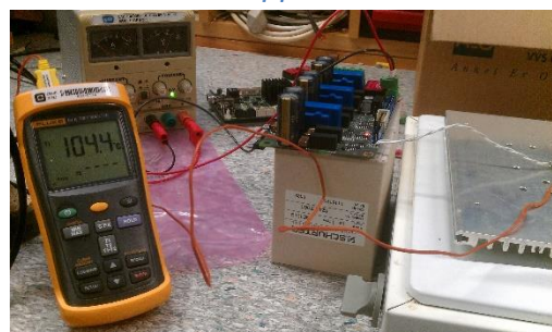
Figure 8.9.5: Heat sink temperature tripping test 104.4 °C, circuit has tripped
