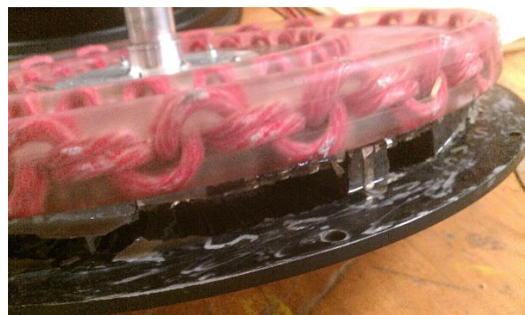
Figure 8.1.2: 2013 axial flux motor loose magnets on rotor plate 2
