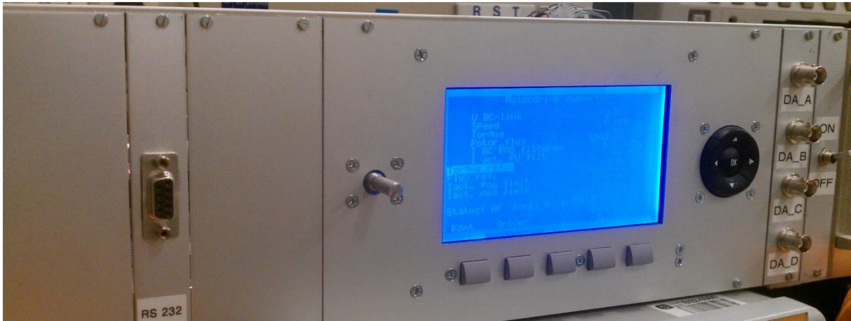
Figure 8.4.3.6: SINTEF FPGA module for inverter control front
