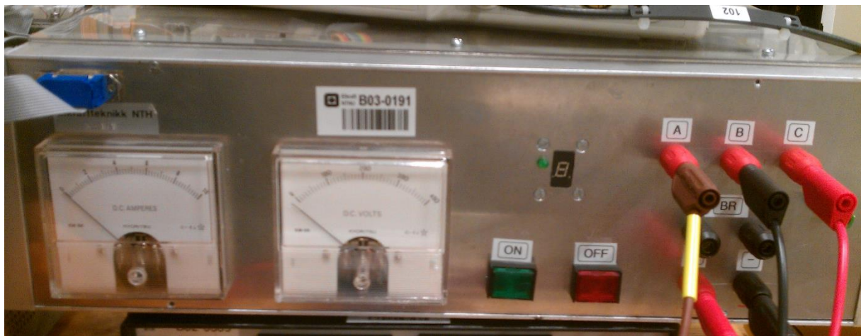
Figure 8.4.3.3: 0-350V 10A, 3U rack, inverter, B03-0191, front
