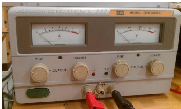
Figure 8.4.3.10: DC source, B02-0360, providing field current to the DC machine
