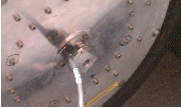
Figure 6.3.1.1: EM1 on DISC-2 urban vehicle encoder mount
