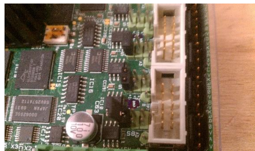
Figure 8.11.3: The three critical jumper connections on the FPGA for correct current measurement
