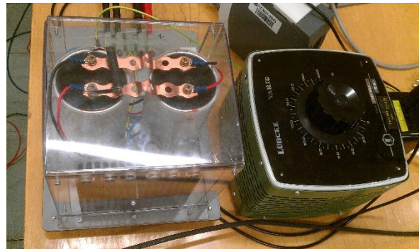
Figure 8.4.3.2: Rectifier, B02-0562, (left) and variac 0-240V, B01-0426, (right)
