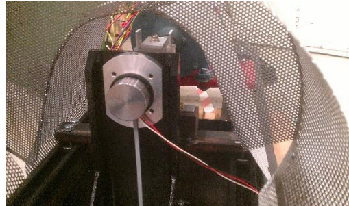
Figure 8.6.1: EC 60 flat motor mounted to the motor test rig
