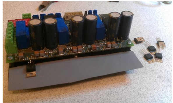
Figure 4.3.6.2: MOSFET soldering process for the inverter circuit board
