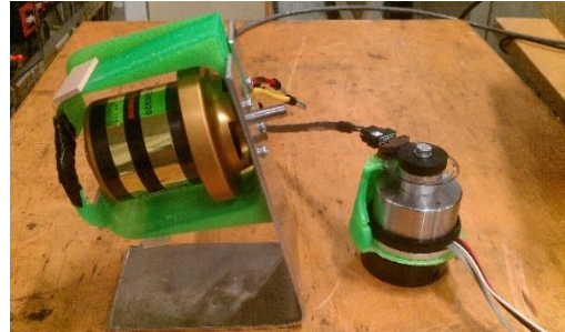
Figure 8.10.1: AXI and EC 60 flat motor with 3D printed plastic mounts for the EM1 encoder
