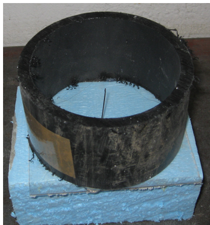
Figure 3-1 Formwork for a pull-out test specimen
