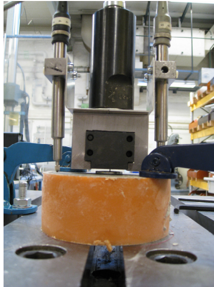
Figure 3-2 Test rig for pull-out tests
