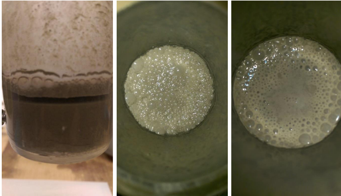
Photo 5: The 2 photos to the left show stable foam, while the one to the right is unstable
