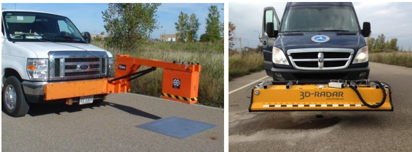
FIGURE 2 ANTENNA ARRAY (LEFT) AND GROUND-COUPLED ANTENNA (RIGHT)
