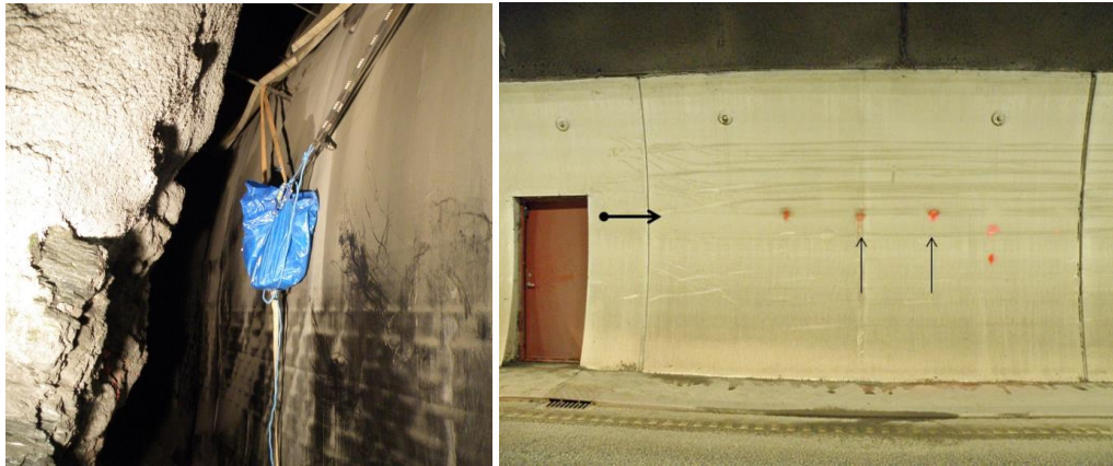
Figure 6a, 6b In-situ field testing in Norway using a step-frequency GPR
