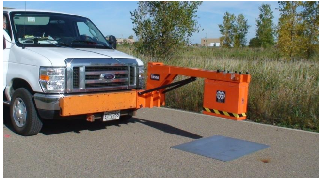
Figure 3 Impulse GPR, air-coupled antenna
