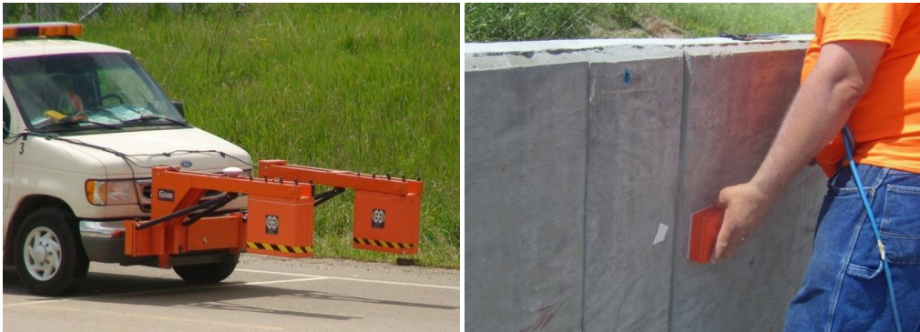
Figures 3a - 3b Air-launched (left) and ground-coupled (right) antennas
