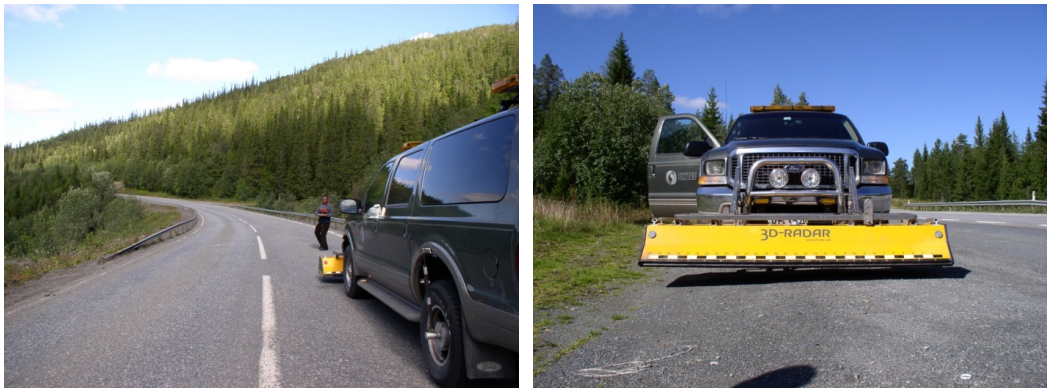
Fig. 2. GPR data collection equipment
