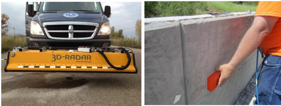
Figure 4 Antenna array (left) and ground-coupled antenna (right)
