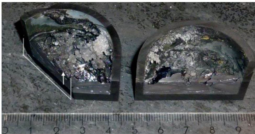
Figure 4.50: Overview photo of the crucible after experiment \text{H}_2\text{O}/\text{CO}_{2.2/2.4} with 0.022 bar steam and 0.024 bar CO. The opposite face to the half cross-section marked by the U-shape is used for microprobe analyzes, and Figures 4.44(a) and 4.44(b) are taken near the arrowhead. A piece of the surface is missing at 3-4 cm on the ruler.
