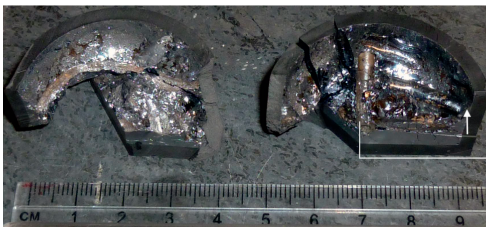
Figure 4.51: Overview photo of the crucible after experiment \text{CO}_{0.1} with 0.001 bar CO in argon. The opposite face to the half cross-section marked by the U-shape is used for microprobe analyzes, and the BSE images in Figures 4.54(a) and 4.49 are taken near the arrowhead.
