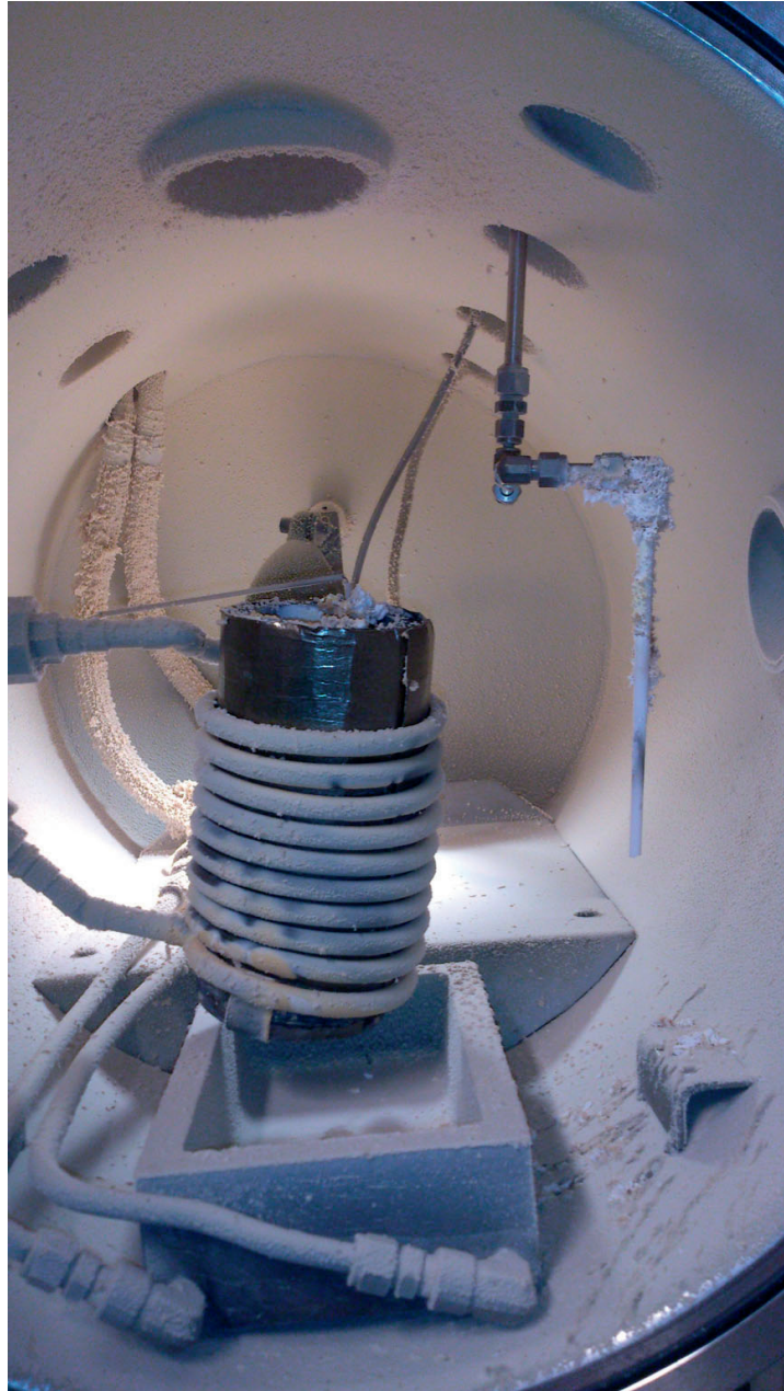
Figure 3.11: Fume deposits in Induction 2 furnace after experiment H 2 O_60.
