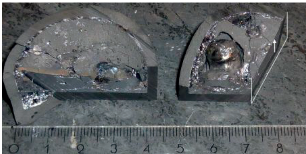
Figure 4.53: Overview photo of the crucible after experiment CO_4.8 with 0.048 bar CO in argon. The opposite face to the half cross-section marked by the U-shape is used for microprobe analyzes, and the BSE images in Figure 4.54(c) is taken near the arrowhead. The ruler measures centimeters.
