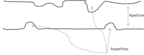
Figure B.4: Representation of a natural fracture with parallel walls with asperities.
