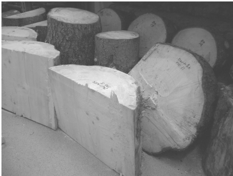
Figure 7-1: Timber logs with large diameters (0.6–0.8 m) during conditioning
