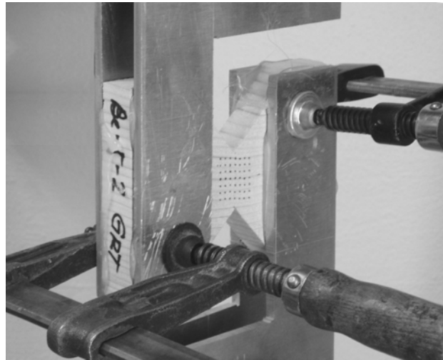
Fig. 10 Arcan specimen marked with an array of dots for deformation measurements
