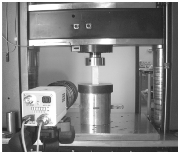
Figure 2: Camera and compression specimen in the loading unit
