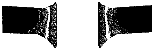
Fig. 15: Final cross-section of target plate perforated by conical projectile (run 300-40) using adaptive meshing and plotted with fringes of accumulated plastic strain.
