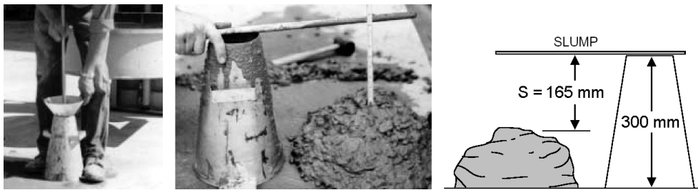
Figure 4.6: Slump measurement is made by placing the slump cone beside the slumped sample and laying the tamping rod across the cone, extending over the specimen. Then the distance from the bottom of the rod to the slumped concrete, gives the slump value S (from [24]).
