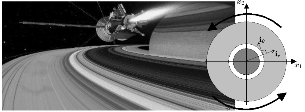
Figure B.5: It is assumed that the velocity profile of the rings of Saturn is \mathbf{v} = v_\theta(r, t) \mathbf{i}_\theta . To the left: An artist rendition of the Cassini spacecraft over the rings [60]. To the right: A schematic top view of the rings and the planet.
