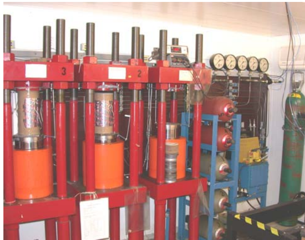
Figure 3-5 Compressive creep rigs equipped with oil pressure accumulators (Note: old measurement system)
