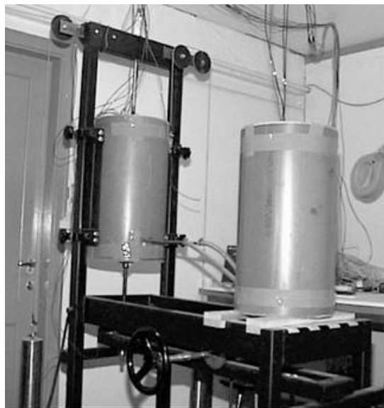
Figure 3-7 Tensile creep rig with dummy specimen (right)
