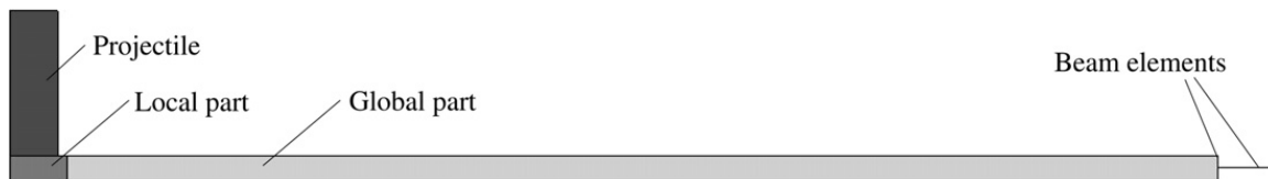
Fig. 17. Finite element model showing the blunt punch, the local part and the global part of the target plate.
