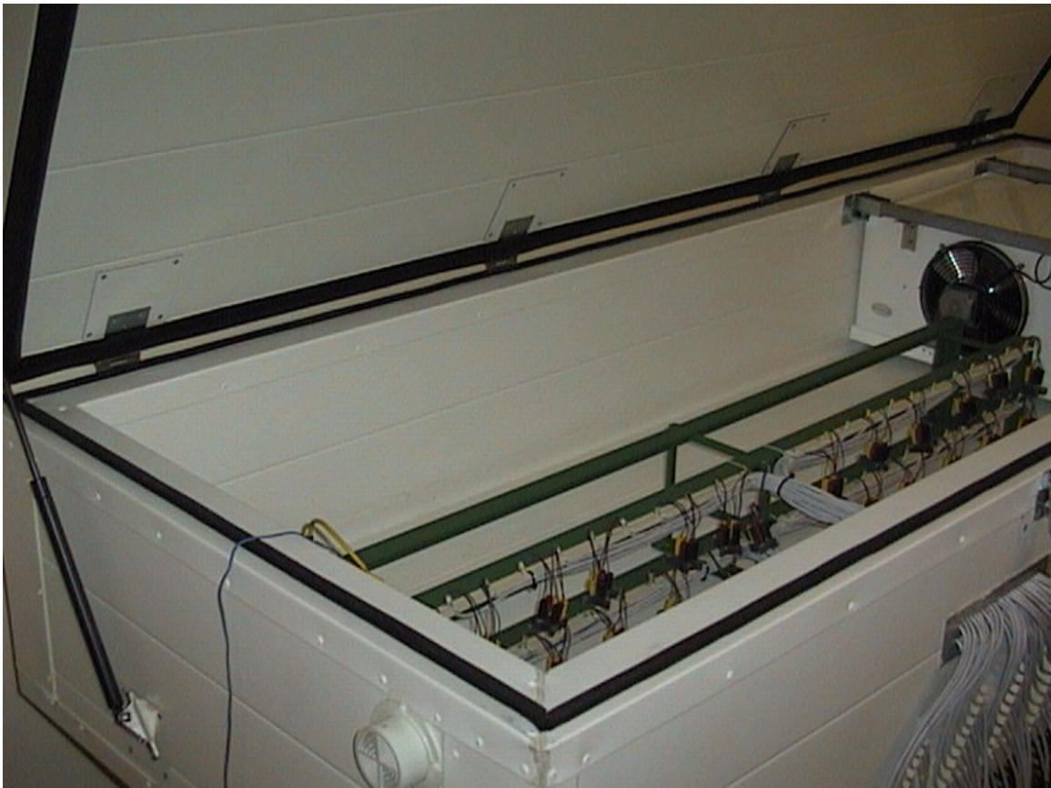
Figure 3. 9 Picture of the Temperature chamber with cabling system
