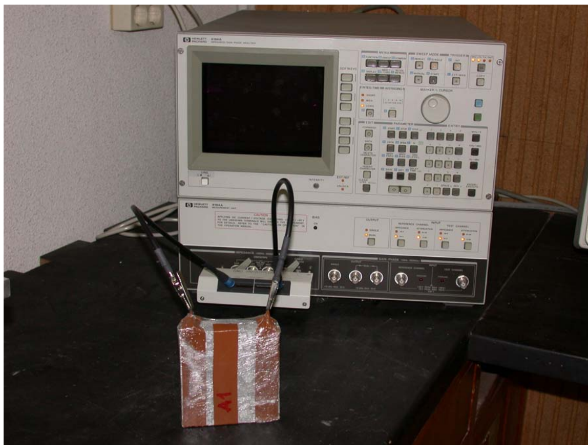
Figure 3. 10 Picture of the equipment for the EIS measurements
