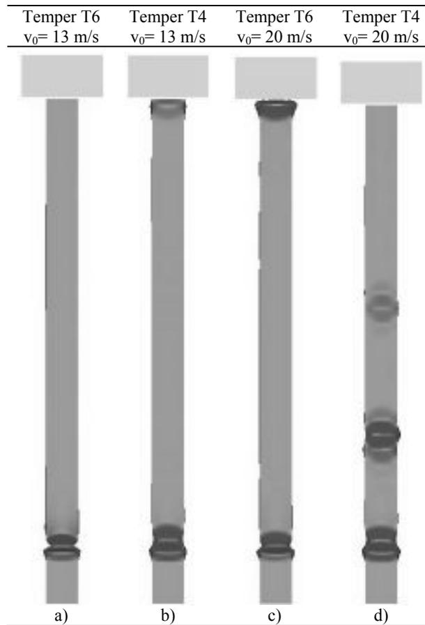
Figure 5-21 Buckling pattern,  $L=1120$  mm and  $h=2.5$  mm.
