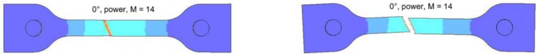
Figure 6.13. Thickness reduction before and after fracture for the 0^\circ simulation with M=14 .
