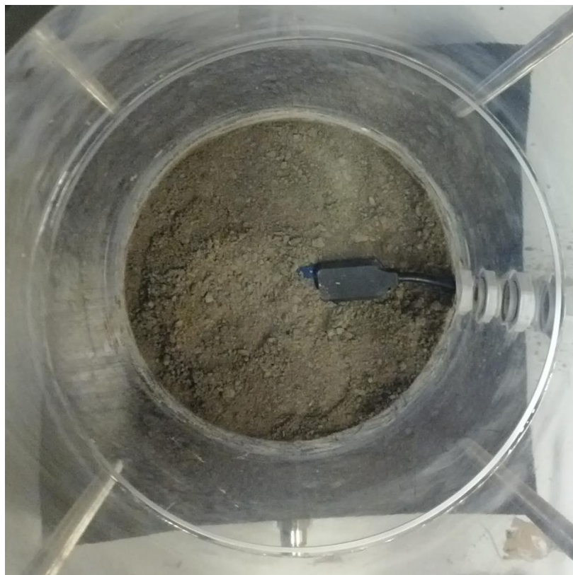
Figure 34 - Installation of sensor
