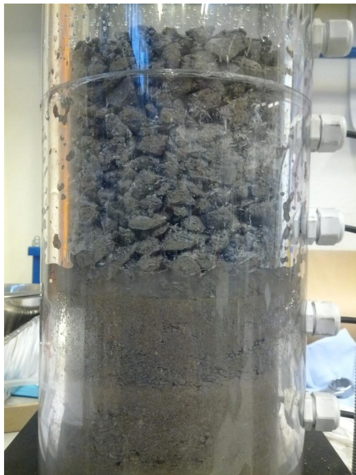
Figure 36 - The cell in the middle of the test. If watched closely it is possible to see the water front approximately halfway down in the fine material.
