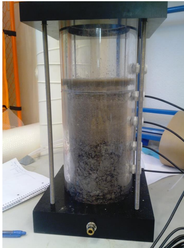
Figure 37 – The cell ready during the second test after the first pouring. Note the small layer of water on top of the fine material.
