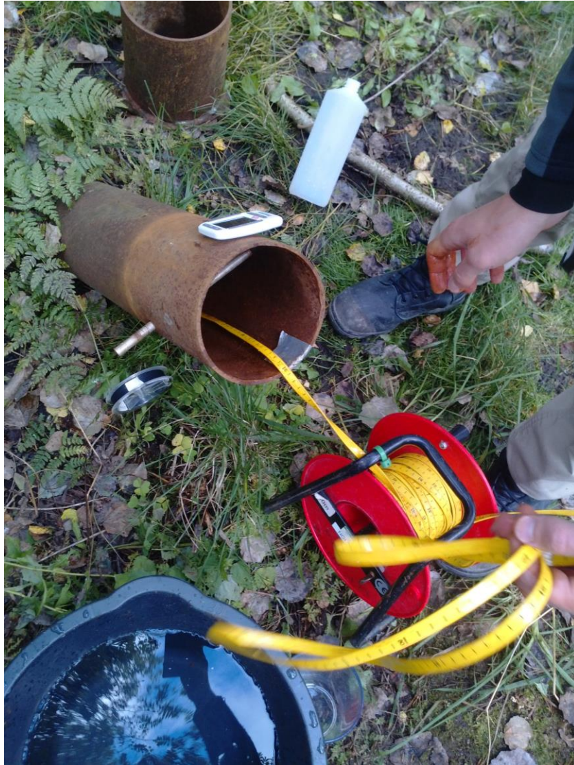
Figure 22 – The setup during testing of well BH5 at Vettakollen. There can be seen water for injection, groundwater level measurement device with a measuring tape, fishing line and a watch in the picture. This well had an angle of 65° with the horizontal plane.
