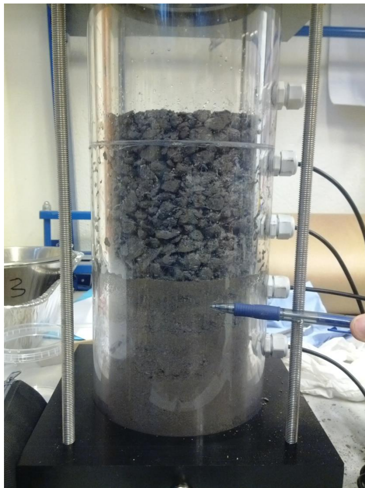
Figure 35 – The full setup after preparing both the fine and coarse material as well as the sensors within the cell.
