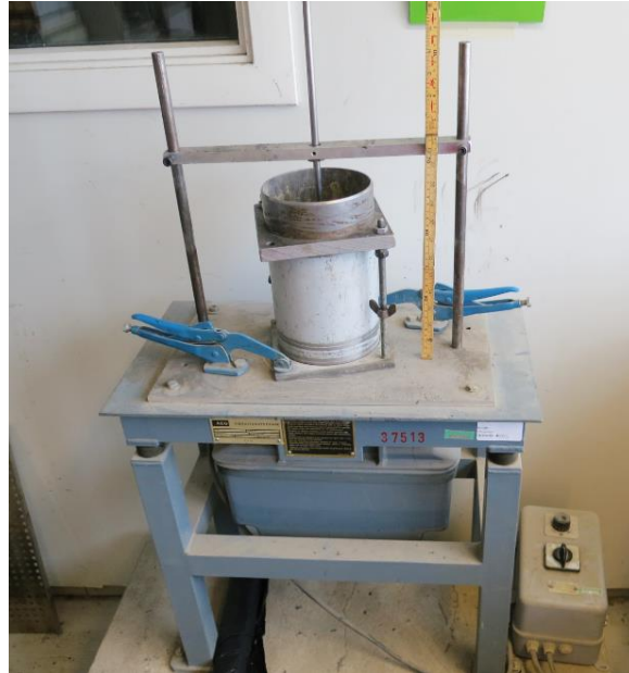
Figure 23: Second layer of material under compaction with a vibration apparatus.
