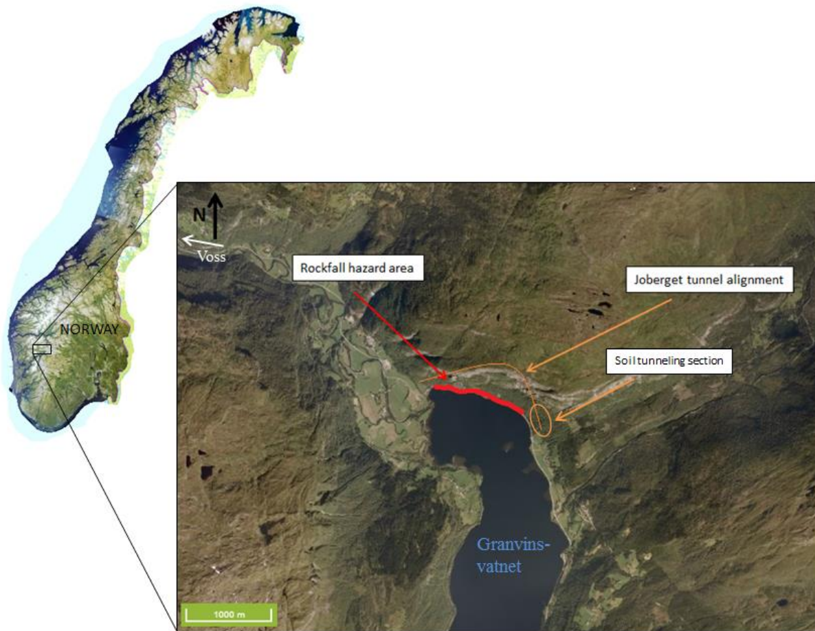
Figure 1: Air photo showing the location of Joberget tunnel. The rockfall hazard area in red and Joberget tunnel alignment in orange are illustrated based on information from NPRA (2013a). The figure is modified after the Norwegian website, norgebilder.no (2013).
