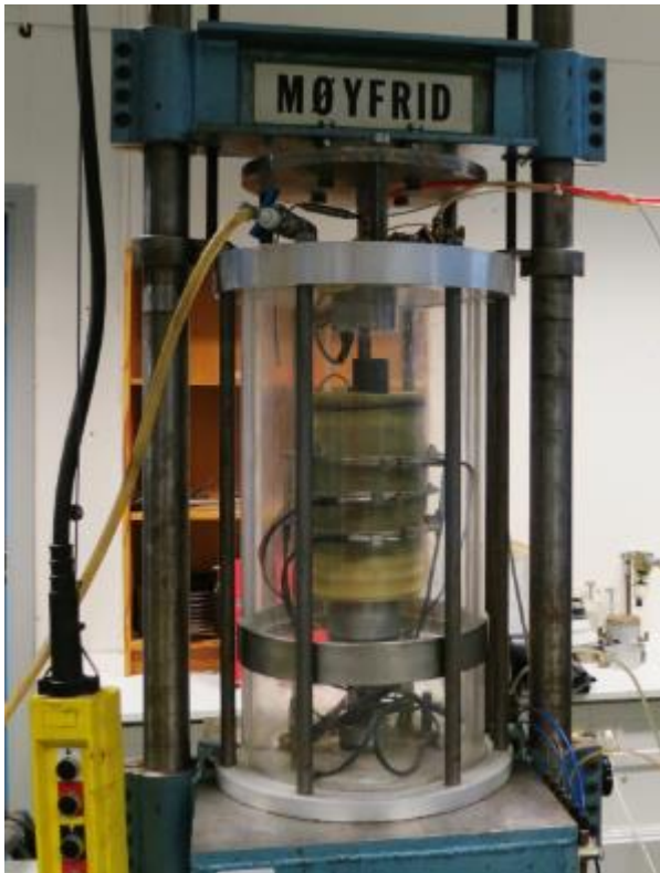
Figure 26: The triaxial apparatus, Møyfrid showing the test specimen inside the chamber with installed LVDTs . This test specimen is constantly loaded with a confining pressure of 50 kPa.
