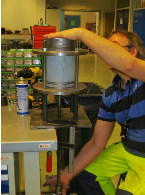
Figure 24: The laboratory technician demonstrates how the material was transferred from the cylinder into the rubber membrane.
