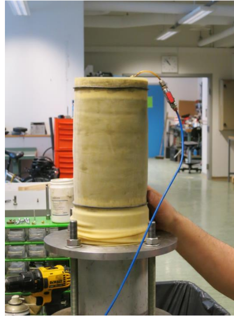
Figure 25: Together with vacuum the material was slowly screwed into the rubber membrane. The black O-rings were placed at the top and the bottom.
