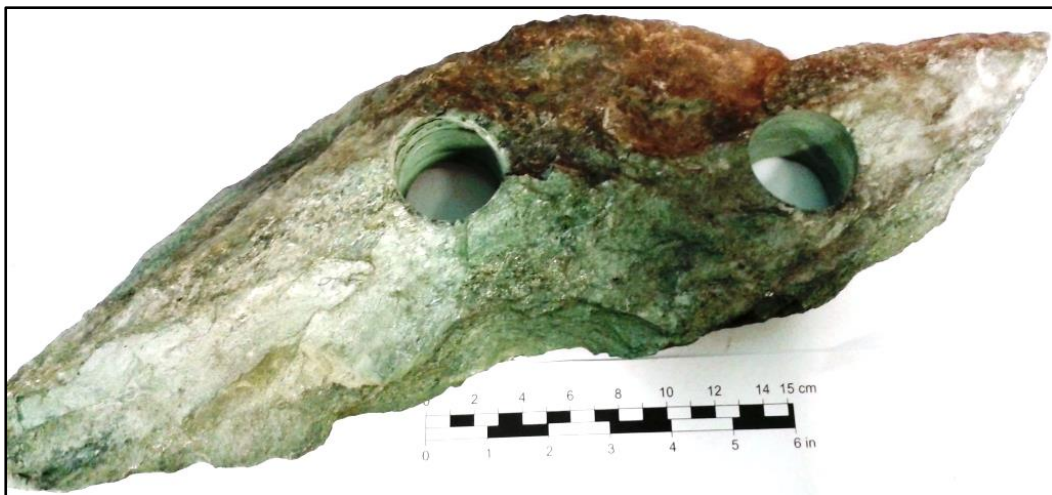
Figure 4-2: Photo of greenschist after core drilling.
