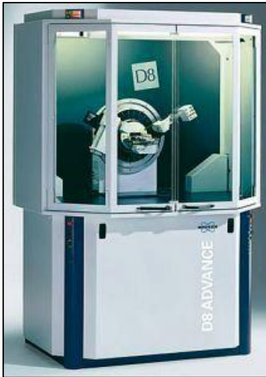
Figure 5-11: Photo of the XRD instrument used for X-ray diffraction analysis, left, a close up of the components of the XRD instrument, upper right (The Bruker Corporation, 2014) and the principal of XRD-analysis, lower right (Nilsen and Broch, 2009).
