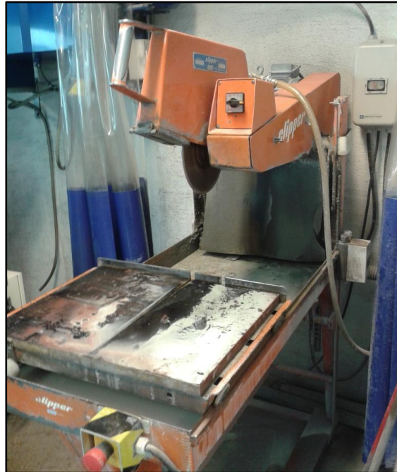
Figure 4-10: Photo of the cutter machine used for cutting of the rock cubes.
