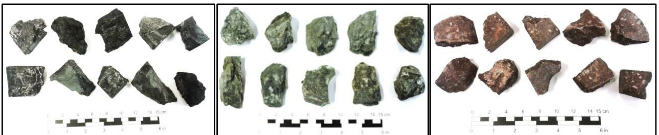
Figure 4-12: Photo of prepared rock pieces for slake-durability testing, from left to right; alum shale, greenschist and tuff.
