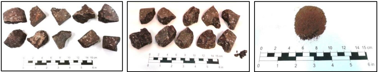
Figure 6-21: Photo of the retained tuff fragments after the testing, left and material which has passed through the drum, right.
