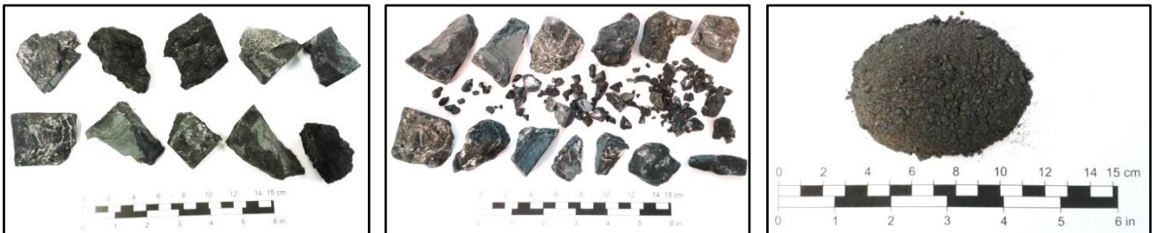
Figure 6-19: Photo of the material before testing, left, retained alum shale fragments after the testing, centre and material which has passed through the drum, right.
