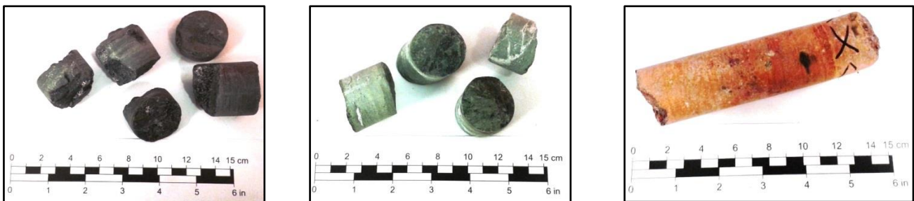
Figure 4-7: Photos of drilled rock cores, from left to right; alum shale, greenschist and tuff.
