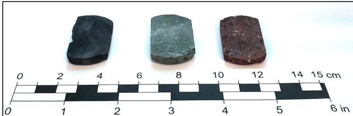
Figure 4-13: Photo of customized rock cores for microscope slides, from left to right; alum shale, greenschist and tuff.
