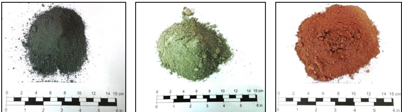
Figure 4-5: Photos of prepared dust powder for free swelling, swelling pressure and XRD analysis, from left to right; alum shale, greenschist and tuff.
