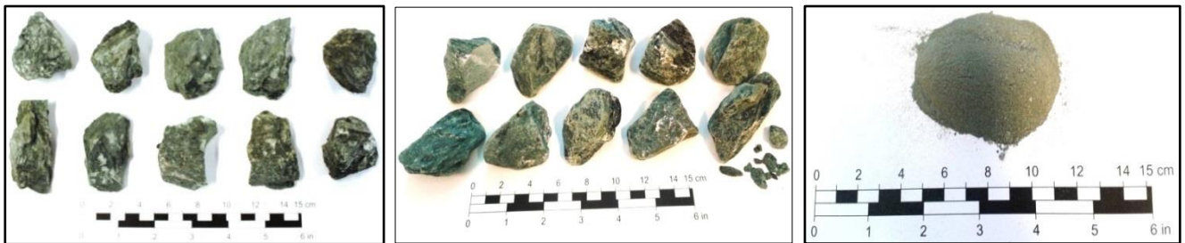
Figure 6-20: Photo of the retained green schist fragments after the testing, left and material which has passed through the drum, right.
