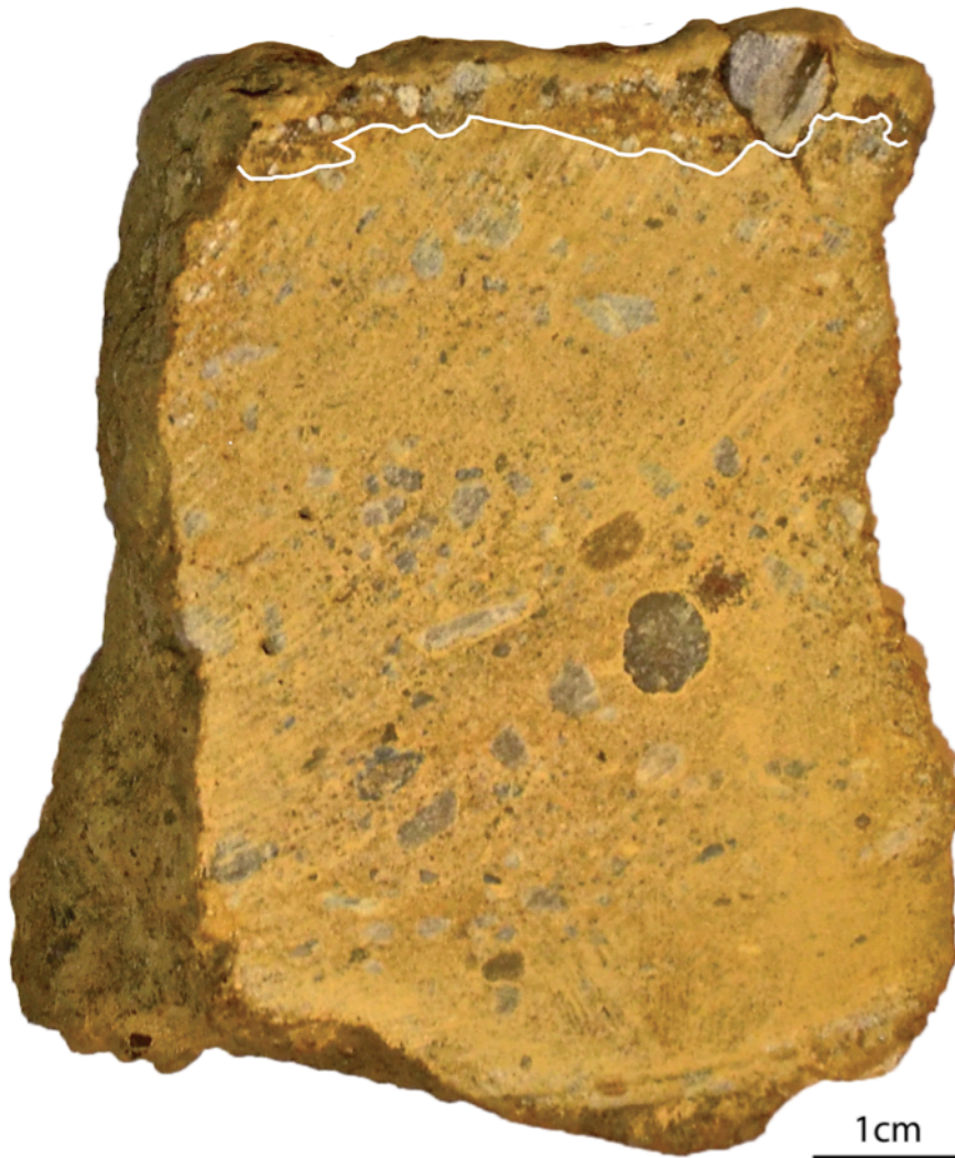
Fig. 16 – Cut section through TSK3 conglomeratic sample, Kovalevskajafjellet. Note the thin clast-supported layer at the top of the sample, carving through the underlying matrix-supported rock. For information, the faint curved marks crossing the sample from the lower left to the upper right are saw scars.
