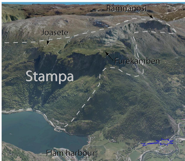
Fig. 1. Aerial oblique view of the unstable slope, Stampa, above the village Flåm ( www.norgei3d.no ).
