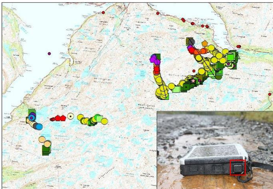
Figure 6 Map of most of the field observation points made during the field work. Different colour codes indicates the lithologies. The photo shows the toughbook. Red square marks the built in GPS(Photo from Henderson and Viola (2011))
