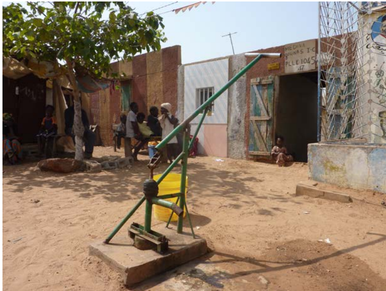
Figure 7.3: Water from the hand-operated Diambar pumps is used for domestic activities like washing and given to animals. The photo is of the site DP9. (Photo: author)
