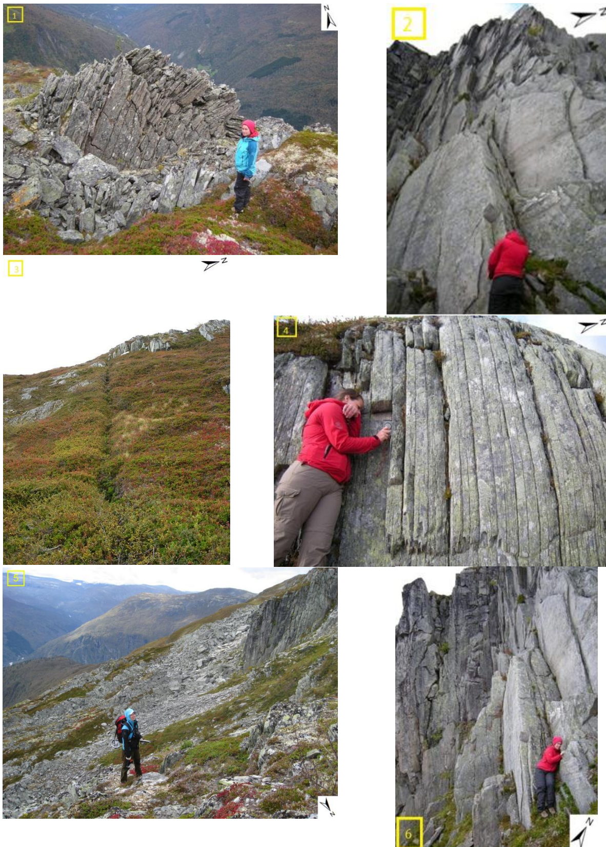
Figure 26 Different pictures taken of Vollan during fieldwork. 1) shows a really good illustration of the toppling failure that is in the area, and this is a mini-scale figure of this. 2) & 6) are taken from the back scarp, it shows clearly that it is really steep, fractured and contains massive quartzite. 3) shows a huge horizontal crack behind the back scarp. 4) is taken behind the back scarp, and the layers are quite thin here, but still quartzite. 5) partly overview of the area, back scarp to the right. Photo taken by the author and Yngvild S. Kvalvik.
