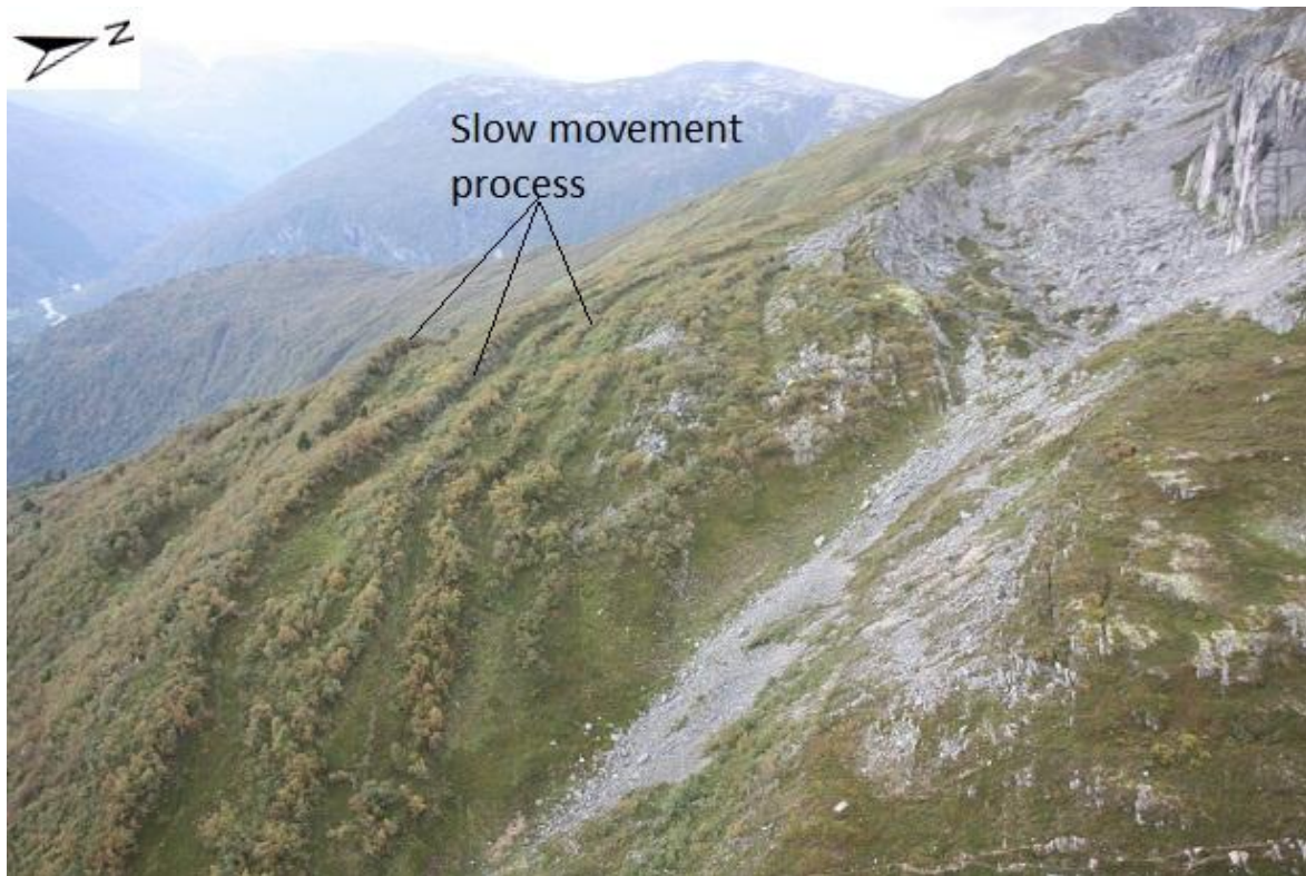
Figure 27 The really slow movement process of the ground is really easy to see in the field and by orthophoto, this picture is taken by T. Oppikofer, NGU with helicopter in August 2011.
