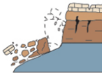
Figure 8 Illustrates toppling failure (USGS, 2006).
