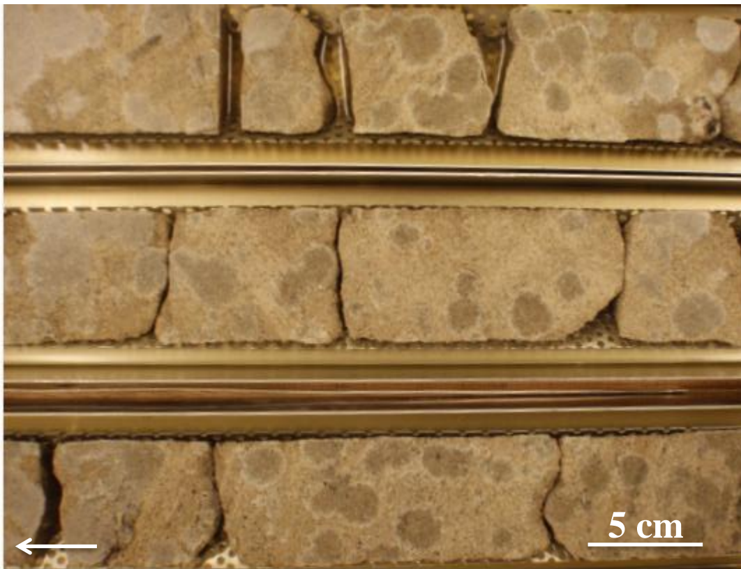
Figure 6-3: The concentric calcite patches as they are observed in the core. The arrow shows the upwards direction of the cores. This section is from 35-37 meters depth.
