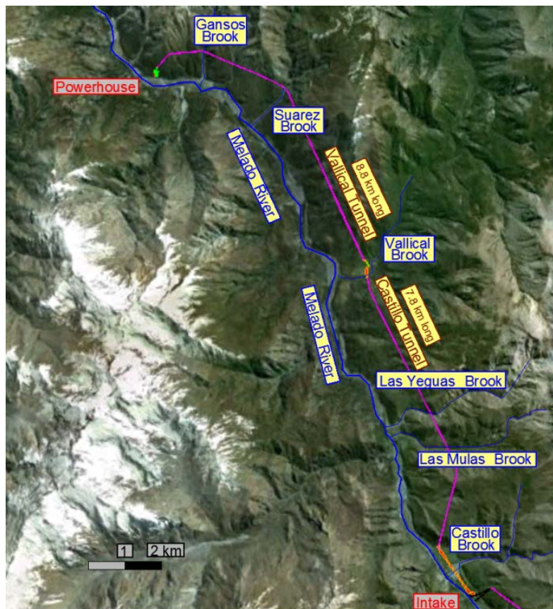
Figure 2-5: Layout of the Melado HPP and its two head race tunnels (Castillo & Vallical).
