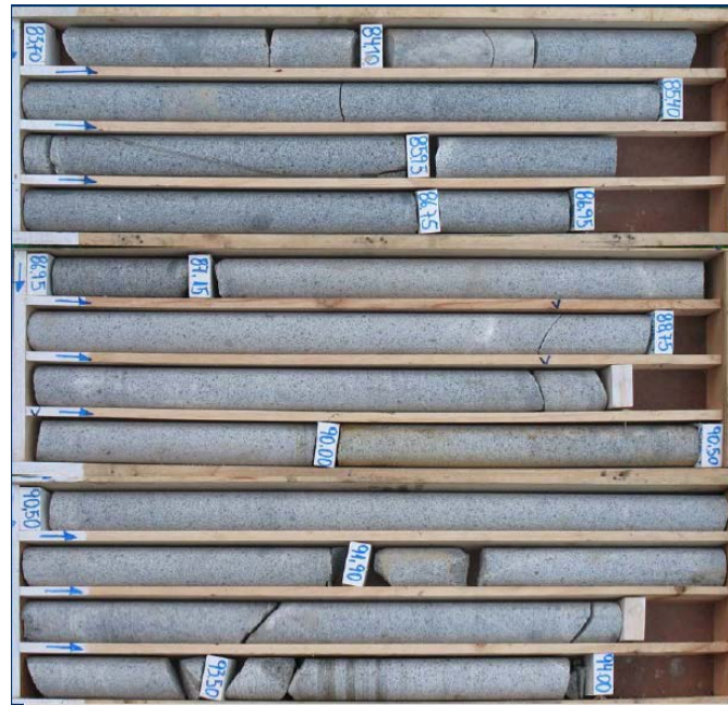
Figure 3-15: Core drilling SCHM-7 (83.7 – 94 m deep)
