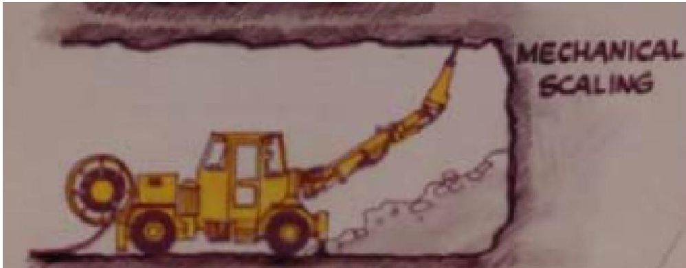
Figure 6.2 Mechanical scaling using drilling rigs
