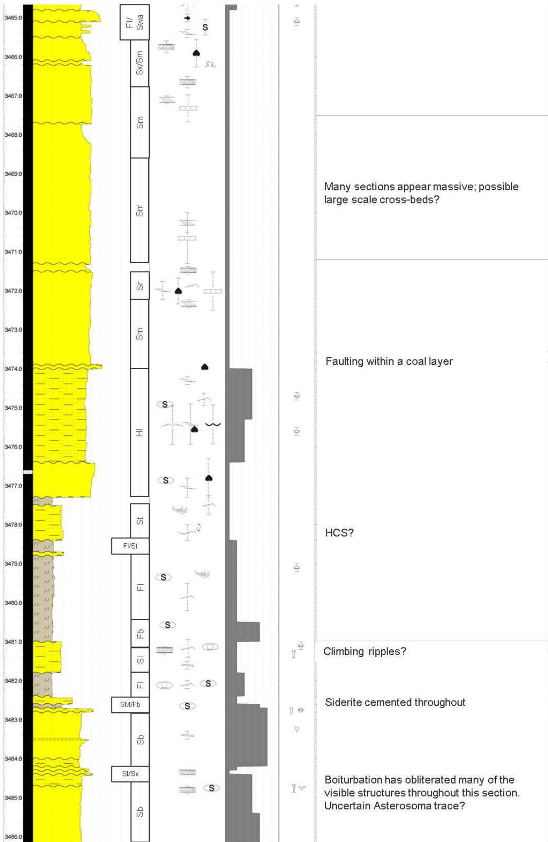
Figure 21: Core log of well 30/9-16, depth 3465 m - 3486,2 m.
