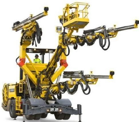
Figur 2.2.2-2 Tre-boms fulldata borrigg Boomer XL3 D (Copco, 2012)
