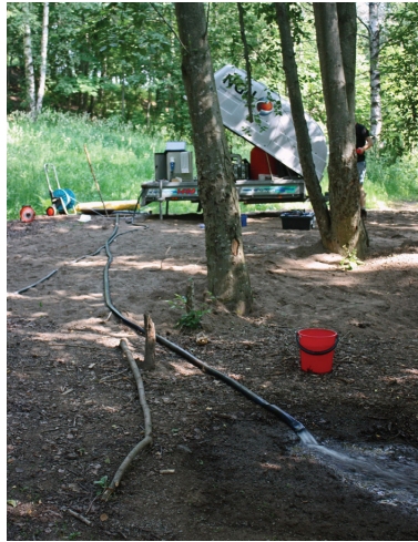
Figure 2.2 Preparations for the TRT with pumping of groundwater at Bryn.
