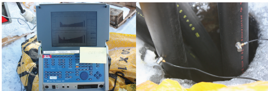
Figure 2.9 Vibration measurements performed with an accelerometer (left) and acceleration sensors glued directly on the collectors with epoxy glue (right).
