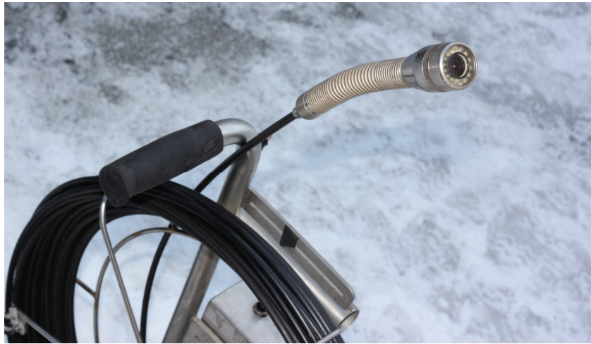
Figure 2.5 Borehole camera used at Lade to visually prove convection in the borehole during TRTs.
