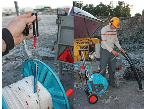
Figure 2.6 VEMCO minilogger and sinker bound to a chord with two meter marks for manual depth determination (left) and temperature logging inside the collector pipe (right).
