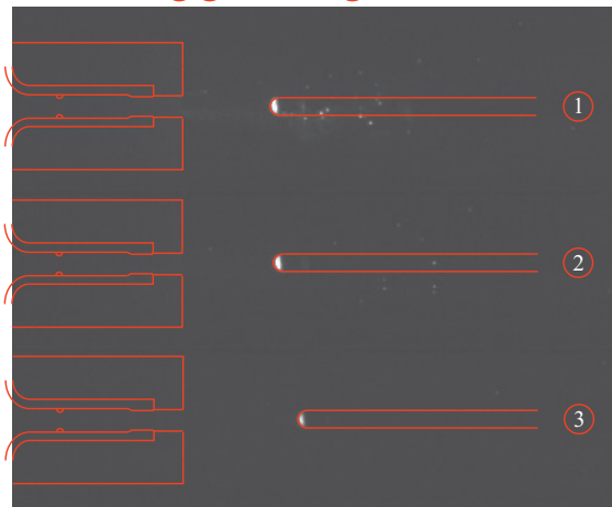
Figure 4.2: A successful interruption with current and voltage measurements, and images of the interruption from CZ and onwards. Contours of the test switch are drawn onto the images.
