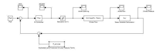
Figure 4.1: Intermediary Block diagram regarding PI controller.
