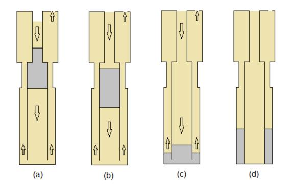
Figure 5.4: Ciment displacement while pumping mud. (a) Cement still inside drill pipe and casing sections; (b) Cement only inside casing section; (c) Cement reaches the bottom and goes to the annulus; (d) Final state with cement inside of the bottom part of the annulus.
