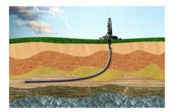
Figure 2.2: Horizontal drilling technique [6].
