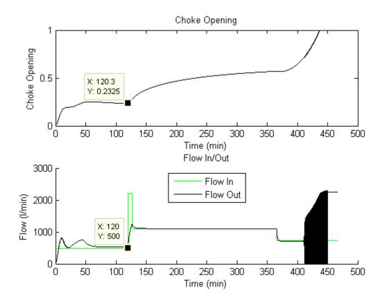
Figure 6.1: Simulation of choke behaviour (top graphic) and flow in and out of the well (bottom graphic). Coordenates pinpointed on both graphics show the transition moment when mud is pumped after cement.
