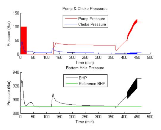
Figure 6.2: Simulation of the estimated pressures at the top and at the bottom (top and bottom graphics respectively).
