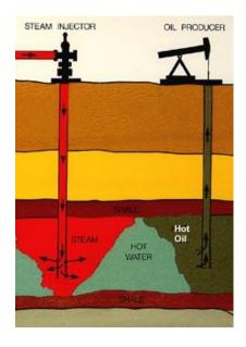
Figure 2.1: Steam injection on the left side that reduces viscosity of the oil through heat on the right side [5].
