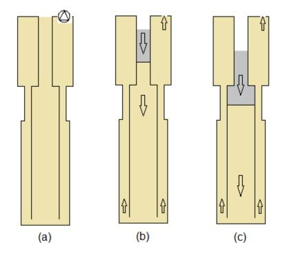
Figure 5.3: Ciment displacement while pumping it. (a) Initial state with no cement; (b) Cement inside drill pipe section; (c) Cement inside both drill pipe and casing sections.
