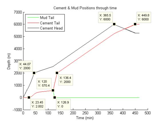
Figure 5.5: Simulation of the behaviour of the fluids inside the well. Pinpointed coordinates show transition states.
