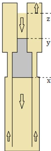
Figure 3.1: Intermediary state with cement between mud.  $x$  – cement head;  $y$  – cement tail;  $z$  – mud tail.
