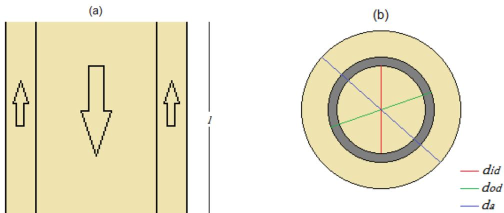
Figure 5.1: Longitudinal (a) and cross sectional (b) views of a well section.
