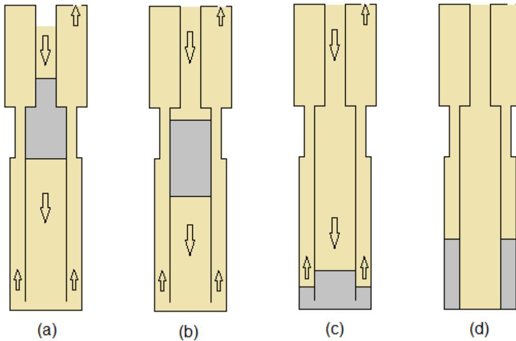
Figure 5.4: Cement displacement while pumping mud. (a) Cement still inside drill pipe and casing sections; (b) Cement only inside casing section; (c) Cement reaches the bottom and goes to the annulus; (d) Final state with cement inside of the bottom part of the annulus.
