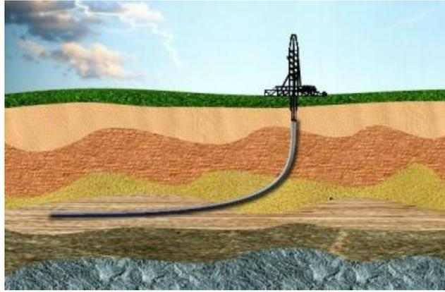
Figure 2.2: Horizontal drilling technique [6].
