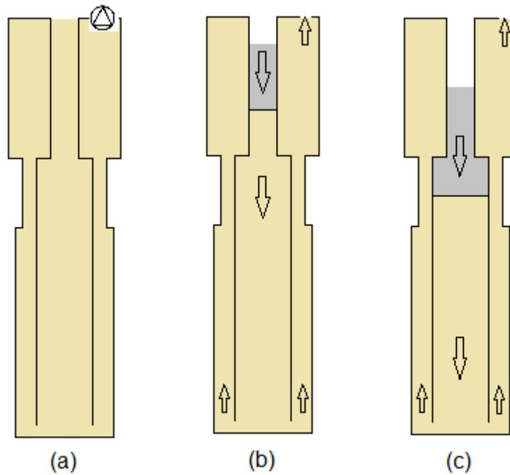
Figure 5.3: Cement displacement while pumping it. (a) Initial state with no cement; (b) Cement inside drill pipe section; (c) Cement inside both drill pipe and casing sections.
