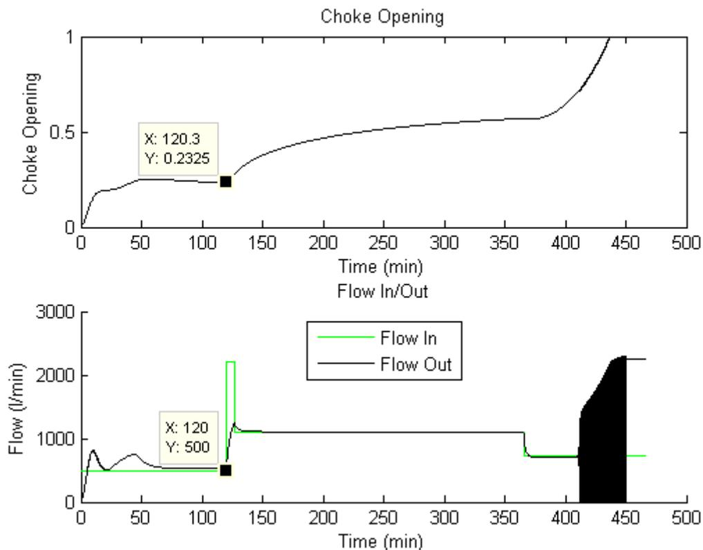
Figure 6.1: Simulation of choke behaviour (top graphic) and flow in and out of the well (bottom graphic). Coordinates pinpointed on both graphics show the transition moment when mud is pumped after cement.
