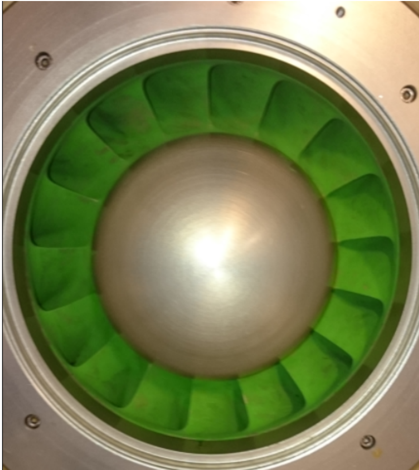
Figure 30: Impeller after application of coating
