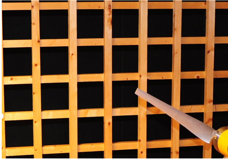
Figure 4.2: Mesh grid installed at the inlet test section. The turbine is not installed during these measurements
