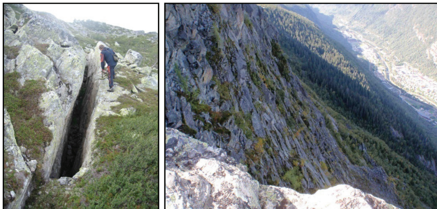
Figure 1.6: Left: Open fracture at edge of top plateau. Right: K1 fractures parallel to valley slope in upper section of the potential instability. (Figures from Loftesnes 2009)
