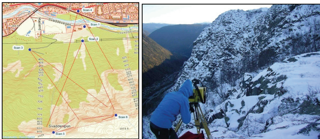
Figure 2.3: LiDAR positions (Left) and ILRIS-3D scanner at location 5 (Right). Locations 1-4 are in the valley floor and location 5 and 6 are at the top plateau. (Figure from Loftesnes 2009)
