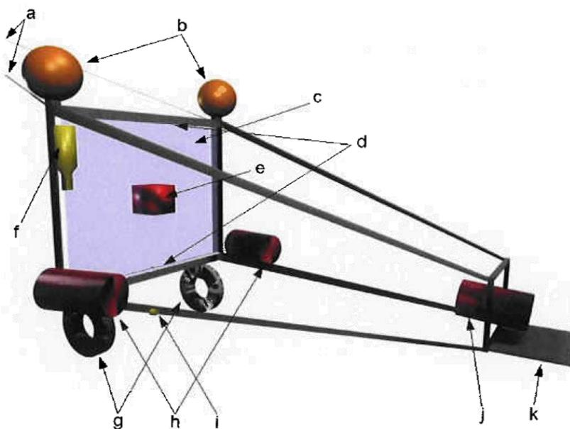
Figure 2.5.1. Schematic description of LVPP that shows the most important features. a=towing cables, b=floatation buoys, c=opening, d=directional light, e=illustrative medusa in the opening, f=transponder, g=steel weight, h=battery packs, i=CTD, j=aluminum casing for video camera, k=stabilizing fin. Adopted from Hetland (2008).
