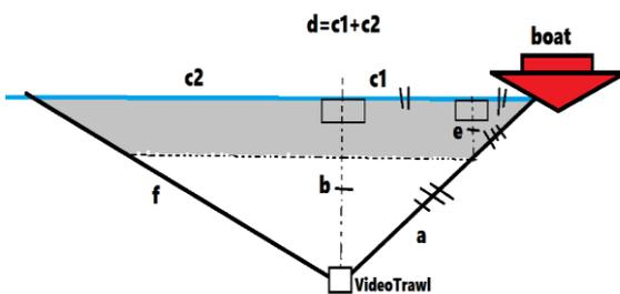
Figure 2.5.2. Visual explanation of how to calculate filtrated water volume.
