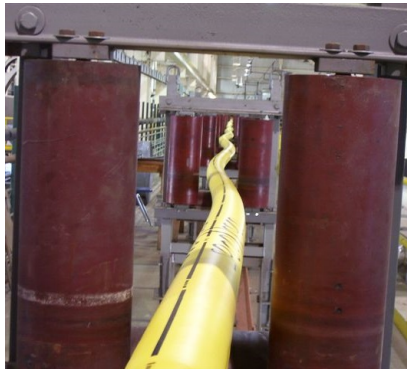
(a) Undesirable deformations of 4.5" umbilical cable during reeling after fabrication
