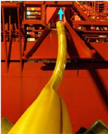
(a) Indication of loop formation at free span between vessel and quay in a flexible pipe load-out operation
