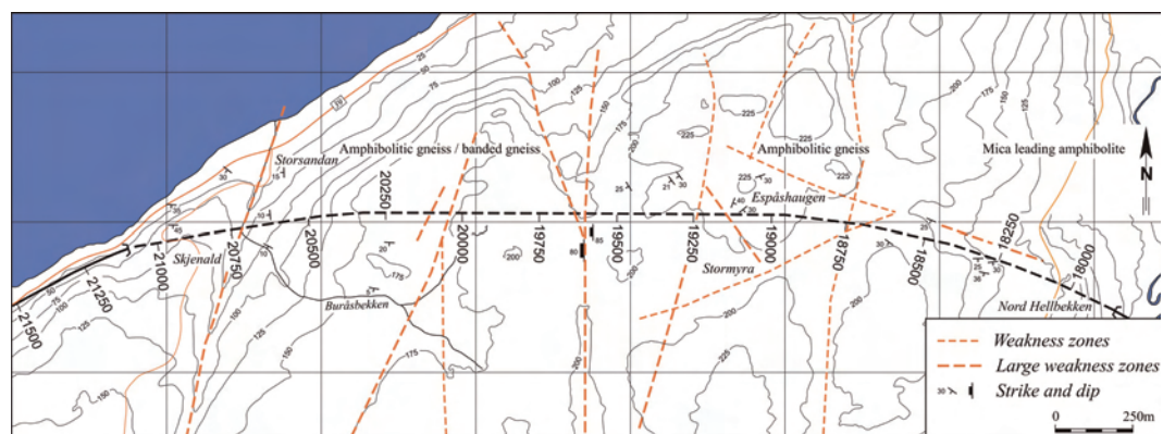
FIGURE 6.11 Simplified geological map with weakness zones for the Storsand tunnel, modified from Hagelia et al. (2001).
