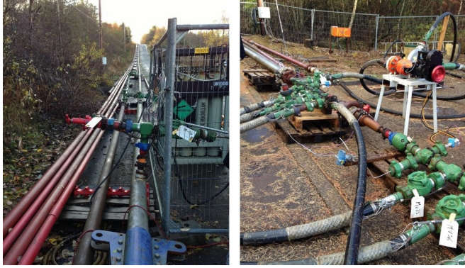
Figure 3.3: Flow-loop setup components for drillstring washout and gas injection (left) and for drill bit nozzles (right).
