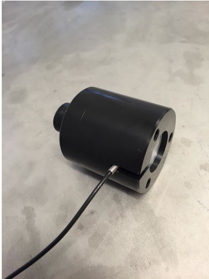
Figure C.4: Gripper 1 sensor house including load sensor.
