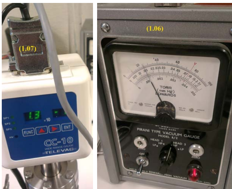
Figure 6 Vacuum pressure indicators
