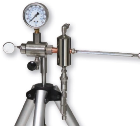
Figure 4.1: The Bureau of Mines dew point meter [5]
