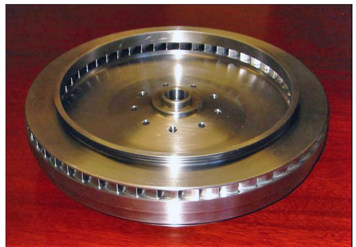
Figure 4. Euler Turbine rotor.
