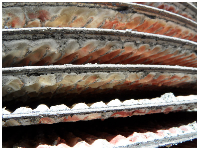
Figure 6. Compact heat exchanger after one month of scale test.
