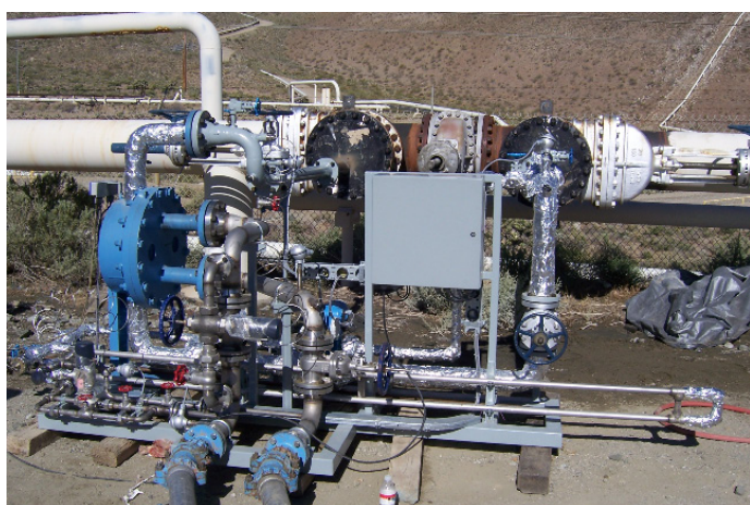
Figure 5. Scale test skid installed at Coso Geothermal.
