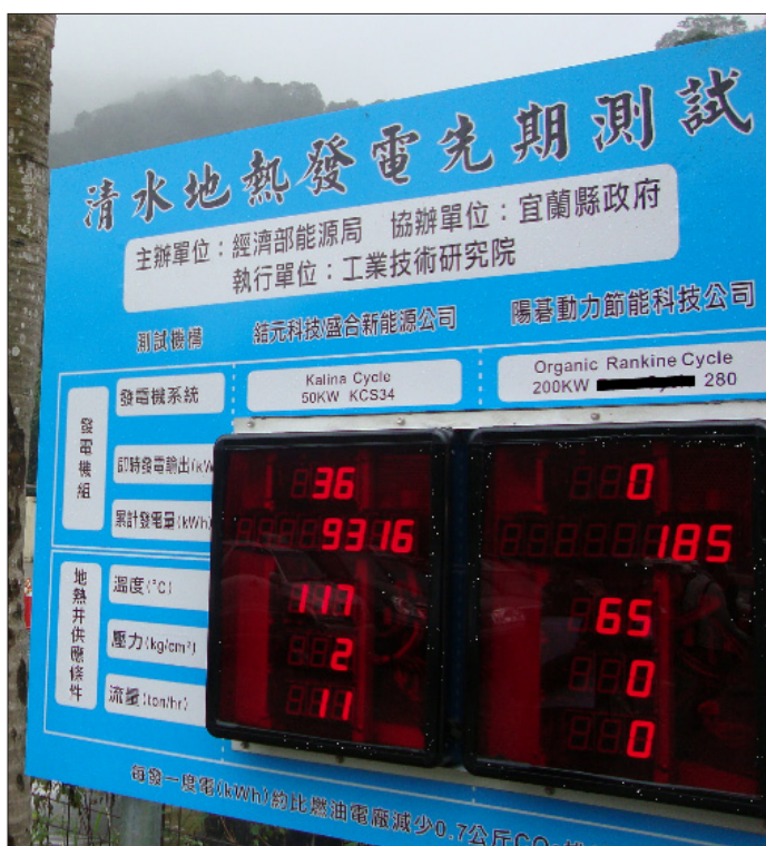
Figure 11. Final results of competition between ORC and Kalina cycles.
