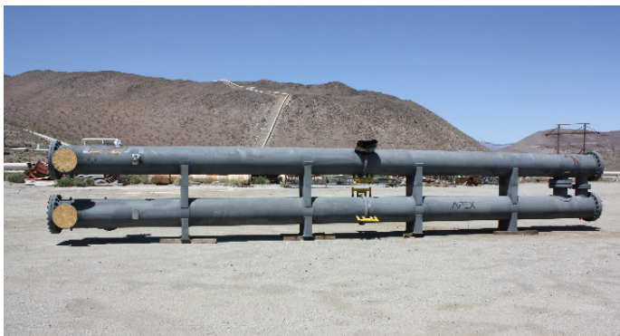
Figure 2. Heat exchanger at Coso Geothermal.
