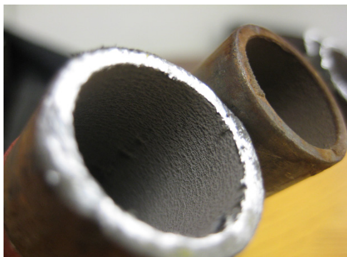
Figure 7. Tubes after one month of scale test.
