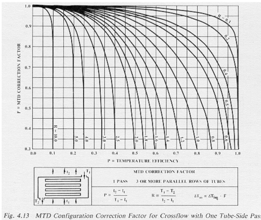
Fig. 4.13 MTD Configuration Correction Factor for Crossflow with One Tube-Side Pass
