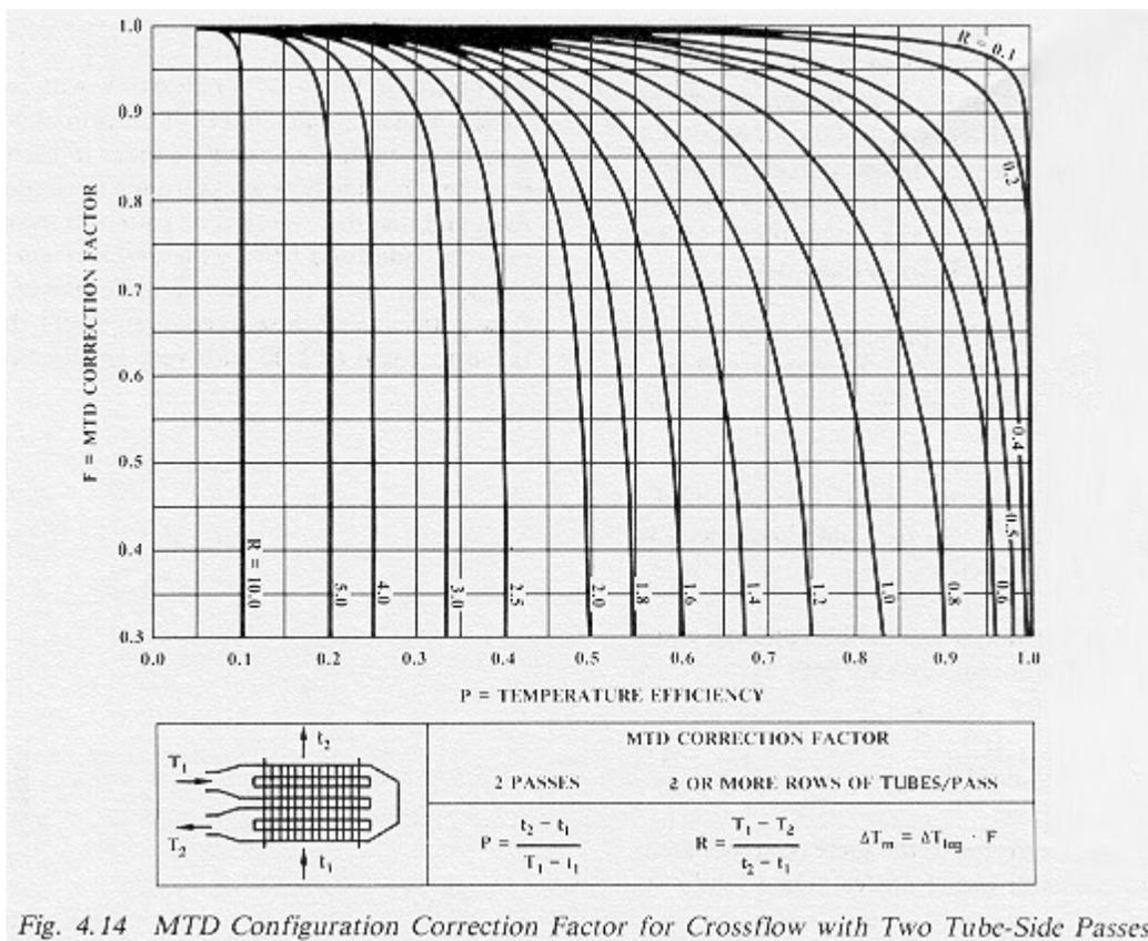
Fig. 4.14 MTD Configuration Correction Factor for Crossflow with Two Tube-Side Passes
