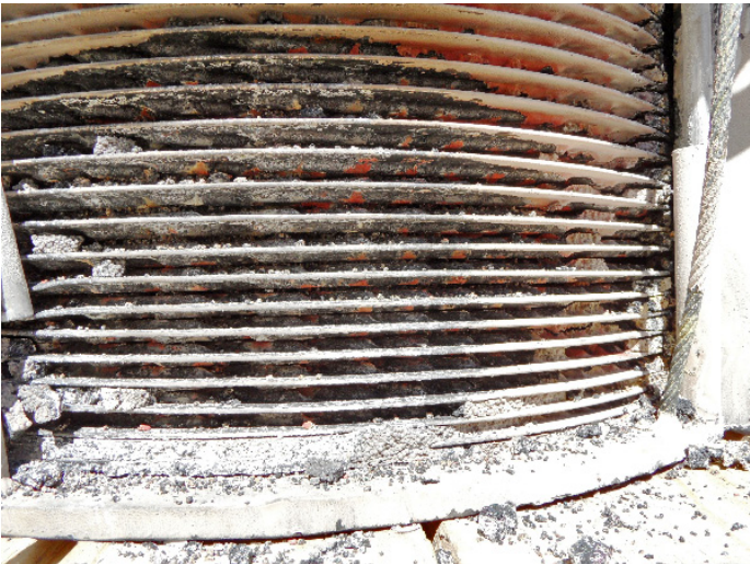
Figure 8. Hydroblast debris in compact heat exchanger after scale test.
