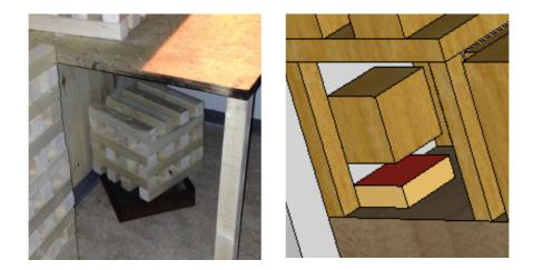
Figure 6-11 Positioning of heptane burner in experiment and heptane burner drawn as "Block Obstruction" in PyroSim
