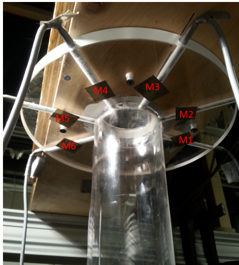
Figure 2.7: Picture of the setup of the microphones around the big jet
