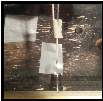
Figure 2.4: Picture of the hotwire above the jet, seen from the 860 mm side view
