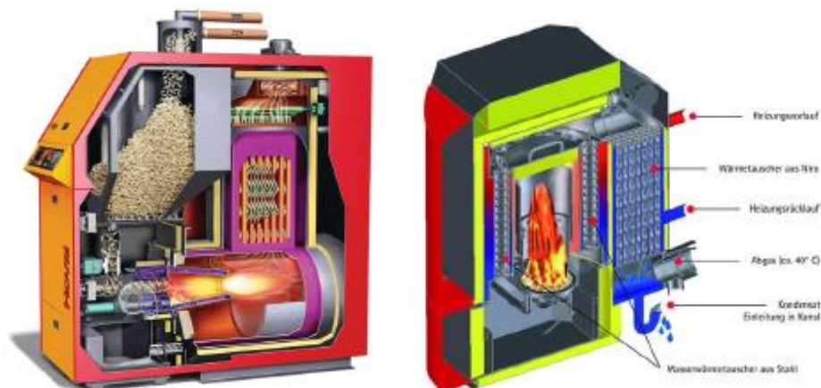
Figure 2.15: Wood pellet boilers [20]
