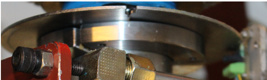
Figure E.0.2: Disc installed at rig to measure rpm, 1 pulse per revolution
