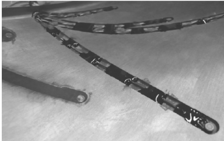
Figure 5.6.4: Procedure to attach pressure transducers along the blade [23]
