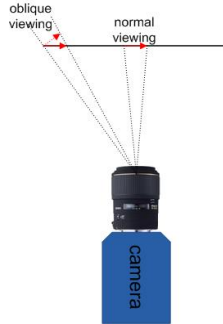
Figure 38 Systematic error caused by viewing direction;
