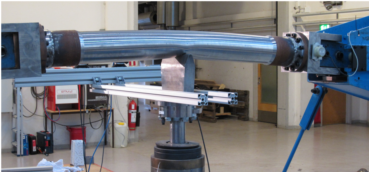
Figure 6.3: Bending of pipe 4.
