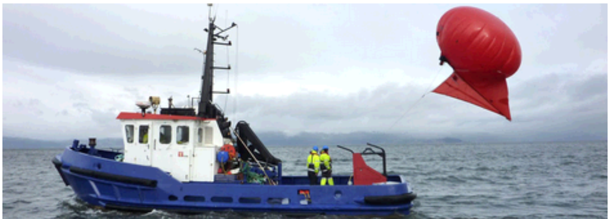
FIGURE 2.10: Picture of the OceanEye system by Maritime Robotics in Trondheim, this is tethered aerostat system that offers a surveillance solution for demanding maritime environment.
