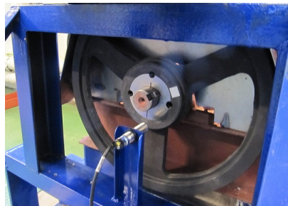
Figure 4.2.9: Optical measurement of rotational speed on turbine
