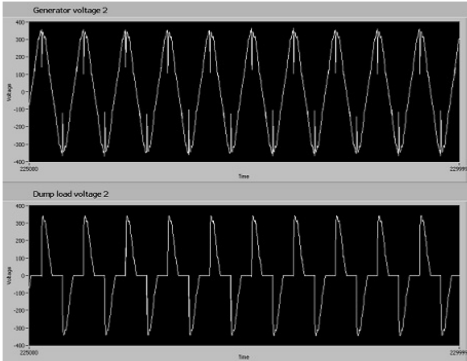
Figure 6.2.2: Generator and dump load voltage. In this situation 6kW dump loads and 1kW consumption loads are connected. The resulting trigger angle is 113^\circ
