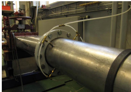
Figure 11: Pressure taps installed perpendicular to the pipe at the entrance of the turbine. Notice the tubes carrying water to the pressure transducer. The when the experiment is running, the tube must be checked of presence of air bubbles. Presence of air bubbles in water in the tube affects the quality of pressure signal from the transducer and gives incorrect differential pressure. The entrained air bubbles are removed from the tubes by bleeding.
