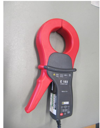
Figure 13: Amp clamp meter used together with Voltech PM3000A
